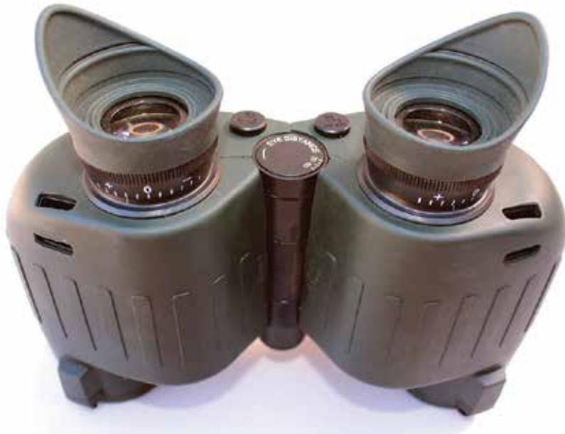
10-power magnification with 30mm objective lens diameters. Its overall dimensions of 165mm wide by 140mm high by 69mm deep and weight of 785 grams make for a very light but compact set of binoculars. Externally, the body of the LRF 1700 is made from ultra-tough polycarbonate Makrolon which is designed to withstand 11G (shock) of impact as well as a Floating Prism System that utilises flexible silicon to absorb severe shock, impact and abuse while protecting the internal glass prisms.
