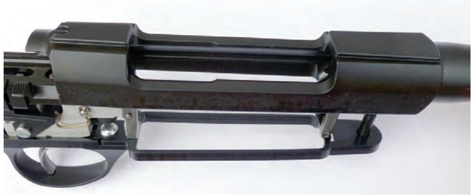
The Sako 85 conical dovetail rail will accept various scope base and ring attachments. However, the Sako Optilock rings and bases are beautifully made and mate with the dovetails perfectly.
