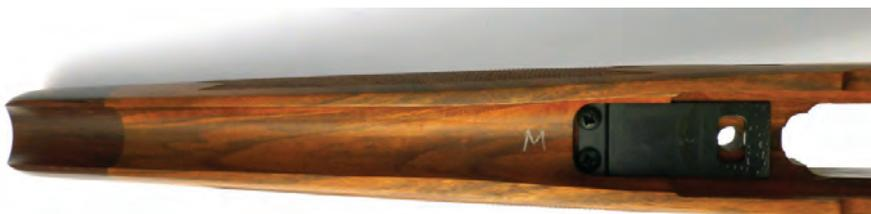
The barrel channel is sealed and very well finished. Note the rosewood fore-end tip and recoil lug bedding arrangement. The barrel free floats.
