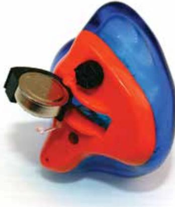
**A standard hearing aid-type battery is easy to replace and is securely housed in the body of the ear protector. SportEAR does recommend that batteries be removed from the units when not in frequent use.**
