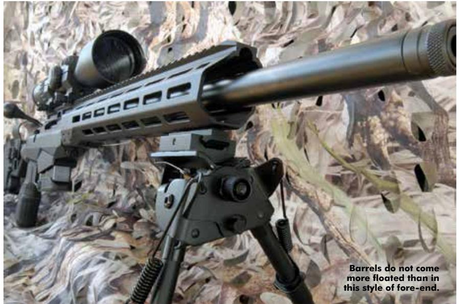
the lower chassis to the action and the M-Lok-designed fore-end cramps onto the sleeve that protrudes from the front of that securing bracket. This fore-end may be swapped out with one of the many aftermarket options available.
