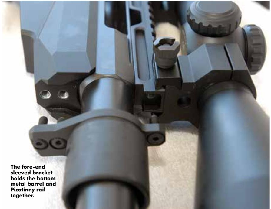
**The fore-end sleeved bracket holds the bottom metal barrel and Picatinny rail together.**
