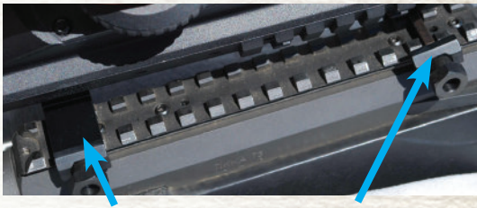
Front Cross Bolt assembly with Plate
